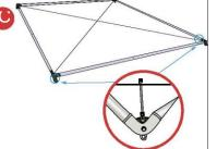
After both ropes are attached, the frame part is formed.
