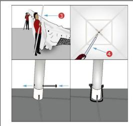
The two legs with no. 3 are attached to the 5 brackets. Then, the middle pole with no. 4 is attached to the slot in the middle, the ower part of the pipe is placed on the steel rope.
