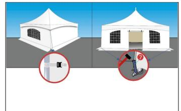
Side curtain columns (tying ropes) are connected from the inside to the frame by means of locking plastics.
