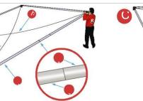
One of the loops at both ends of the steel rope is inserted into the hooks on the triple elbows located at the corners of the formed square. After one loop of the wire rope is attached, one side of the frame is lifted into the air to attach the
